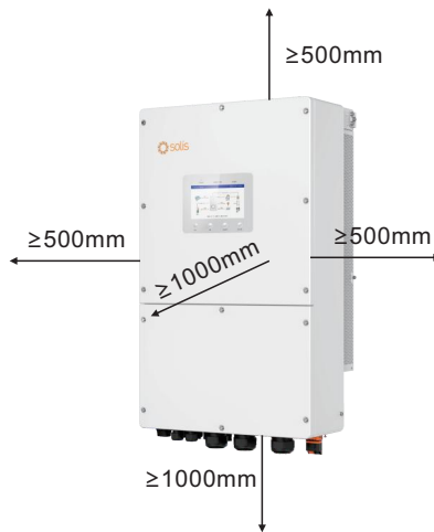
Figure 3.5 Inverter Mounting Clearances
