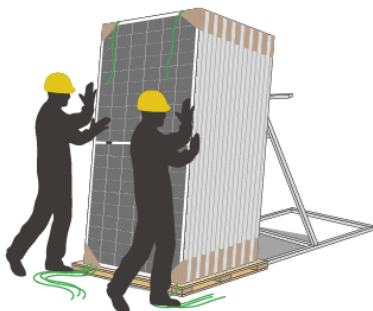
7) Cut off the remaining packing belts so that the modules rest on the stand supporter.
