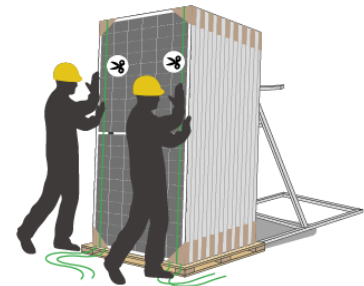
6) When there are 1-2 vertical packing belts remaining, push the module gently to tilt toward the stand supporter.
