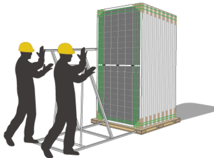
4) Place the stand supporter from the glass side.
