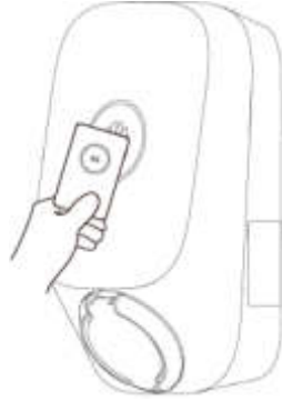
Figure 6-2 Charging by card swiping
