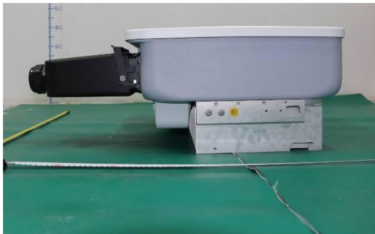
Photo-2: Side view (and second protective earthing screw)
