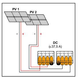
$PV\ 1\ (I_{\text{ccmáx}}) = 18,75\ A/PV\ 2\ (I_{\text{ccmáx}}) = 18,75\ A$
