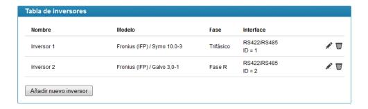
If the inverters are single-phase in a three-phase installation, it is also possible to indicate in which phase each inverter is connected.
