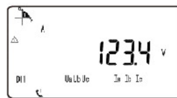
Voltage on A phase
